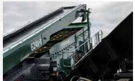
Using two separate screenboxes allows for a lighter built box resulting in more energy for screening. This, coupled with independent settings for each box result in increased screening efficiency.
