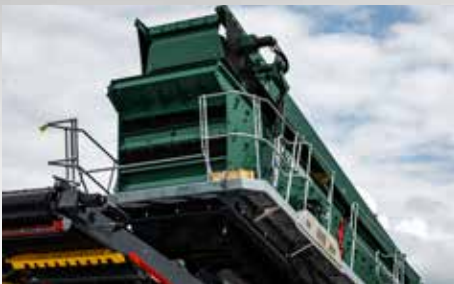
The 624s-t is the largest track mobile screen in its class with a total 6720mm x 1830mm / 24' x 6' screen size, and hopper capacities up to 10m 3 (13.1yd 3 ).
